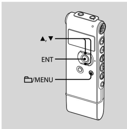
You can erase unwanted messages, retaining all other messages when the IC recorder is in the stop or playback mode. When a message is erased, the remaining messages will advance and be renumbered so that there will be no space between messages.
