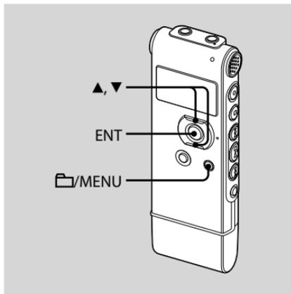
You can set the scanning sensitivity when presetting FM radio stations. The scanning sensitivity is set to "HIGH (SCAN H)" when you purchase the IC recorder.
