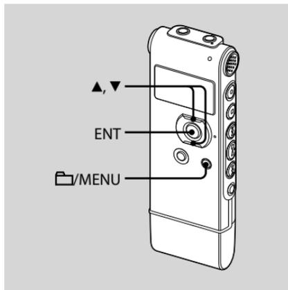
You can set the microphone sensitivity in the menu when the IC recorder is stopped or is recording. The microphone sensitivity is set to “HIGH (H)” when you purchase the IC recorder.
