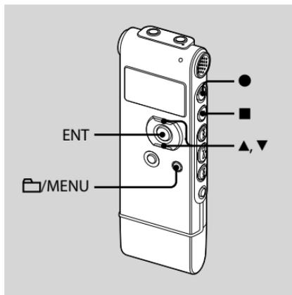
You can set the VOR (Voice Operated Recording) function to “ON,” to make the IC recorder start recording when the IC recorder detects sound, and pause when no sound is heard, eliminating recording during soundless periods. The VOR function is set to “OFF” when you purchase the IC recorder.
