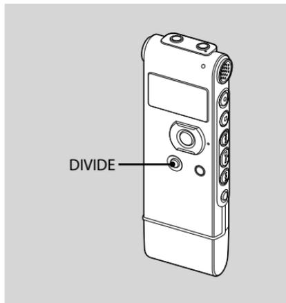
You can divide a message during recording so that the message is divided into two parts, and a new message number is added to the newer part of the divided message.
