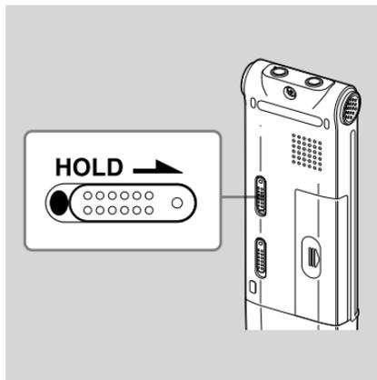
To prevent accidental operation, slide the HOLD switch in the direction of arrow in the recording or playback mode. "HOLD" will appear indicating that all the functions of the buttons are locked.
