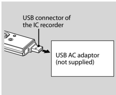
You can connect the IC recorder to an AC outlet using a USB AC adaptor AC-U50A/AC-U50AD (not supplied).
