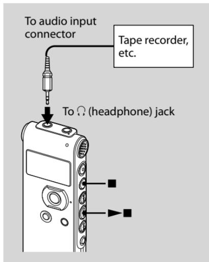
To record the sound of the IC recorder with other equipment, connect the ♪ (headphone) jack of the IC recorder to the audio input connector (minijack, stereo) of other equipment using an audio connecting cable\*.
