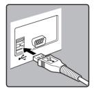
3 Make sure that the recorder is stopped, and then connect the USB cable to the connecting port on the hottom of this recorder
